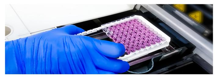
Sandwich ELISA is the most commonly-used ELISA format, which uses matched antibody pairs for capture and detection to enable specificity and sensitivity for the analyte of interest from complex mixtures such as biological samples. The Sandwich format enables superior specificity compared to either a direct or indirect ELISA because there are two distinct analyte-binding antibodies. Each of the antibodies are able to recognize a different antigenic epitope, preventing competition.
