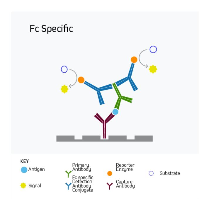
**Figure 3:** Fc and  $F(ab')_2$  specific antibodies can be used to "orient" an assay towards a particular region of the partnered antibody in cases where particular epitopes may need to be preferentially bound in a particular order or direction.
